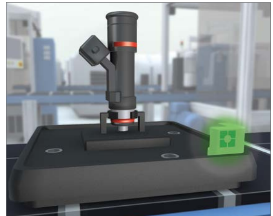
Figure 2: When a build pallet is utilized, RFID tags are permanently mounted to the pallet to enable traceability.
