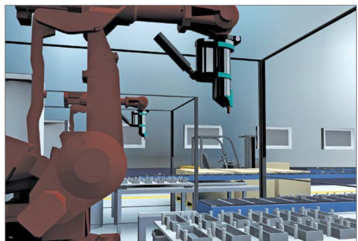
Figure 5: Modular automation sub-systems such as End-of-Arm tooling (EOT) benefit from automated set-up parameters, usage, maintenance, and component matching.
