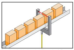
The self-contained thru-beam shown is easy to install. The sensors's rigid construction means that its emitter and receiver are always in alignment and it needs only one cable and no auxiliary electronics. If it's a laser version, it can see through dirty environments, and the one-piece housing conserves space.
