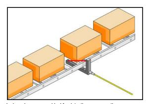
L-shaped sensors are ideal for detecting cases or other square objects on a conveying system. It can be used to see the leading edge of a case or package to initiate glue control, open flap detection, or other gating operations for package inspection.
