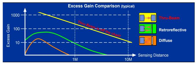
Self-contained laser thru-beam sensors have superior excess gain characteristics over such sensing modes as retroreflective and diffuse. Not only are laser thru-beams very accurate, their high excess gain enables them to maintain their accuracy in the type of harsh environments that would degrade that of most conventional sensors.
