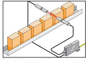
Traditional thru-beam sensor using fiber optics involves comparatively complex setup, including tricky calibration, multiple cables, and multiple components. This makes for longer setup time and a less robust overall configuration during heavy, vibration-prone production cycles.
