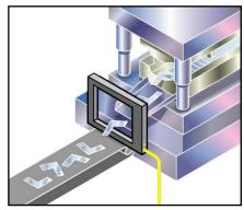
In this example, a dynamic optical window error proofs a progressive die program by making sure each finished part exits the die correctly. This also simultaneously protects the die from double hits by making sure each part is off the die and the press before the next hit.
