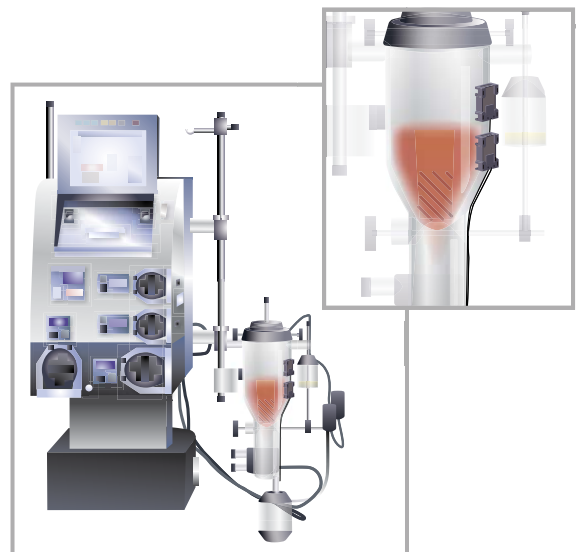
Balluff's Smart Level technology was the device of choice for monitoring blood levels in a disposable blood collection container.
